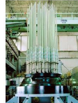
PWR reactor vessel Closure Head
